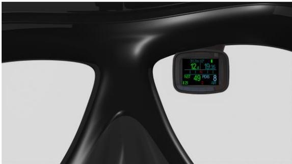
precision near-eye optics, this "floating" display creates a screen image that appears at a virtual distance of approximately 3ft/1m, making it easy for divers to monitor their dive data without losing eye contact with their surroundings, or having to constantly refocus.
